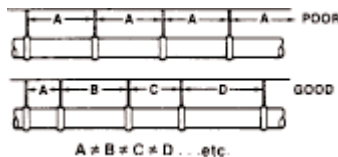
Figure 2: Specify hangers to be installed at uneven intervals to minimize pipe vibration problems
